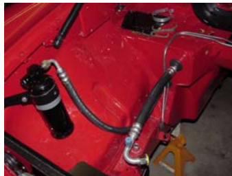
Dryer and hose arrangement
